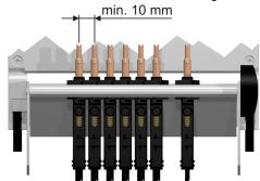
Possible adjustment between base plate and current fingers:
