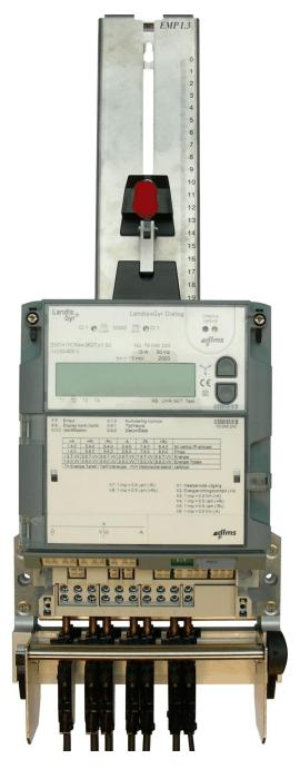
The EMP 1.3 Quick Connection Device is used together with Electricity Meter Test Systems, and is especially recommended for situations where the time factor is of importance. It enables electricity meters to be mounted and connected rapidly for the purpose of their adjustment, test and verification.
