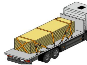
Direct lashing with tie-down lashing
