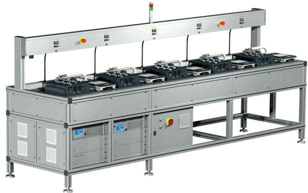
Example of test bench for the calibration of 5 single-phase DC electricity meters
