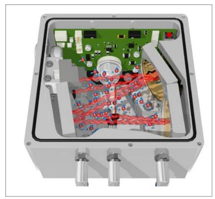
Figure 4. Gas measurement cell
