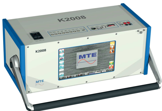
K2008, Three-phase comparator, accuracy class 0.005
