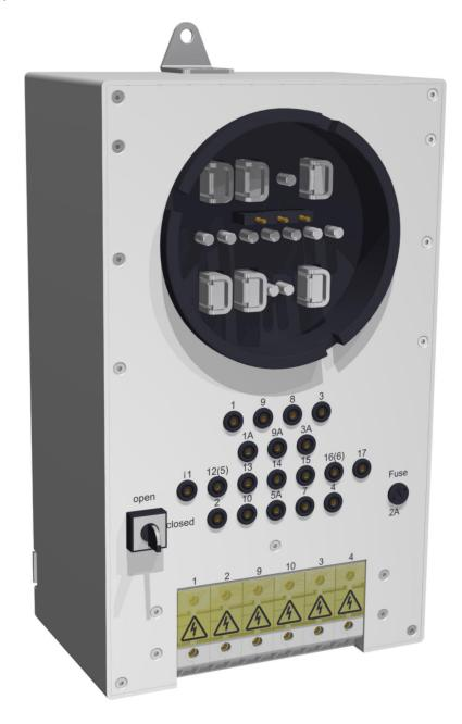
The QCD Form S Universal Quick Connection Device is used together with electricity meter test systems, and is especially recommended for situations where saving time is important. The device enables ANSI socket meters to be mounted with a motorised closing mechanism and connected rapidly for the purposes of adjustment, test and verification.
