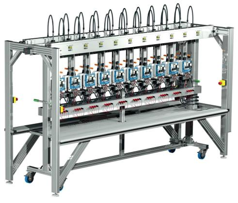
Example of an automatic three-phase test system for 40 positions
