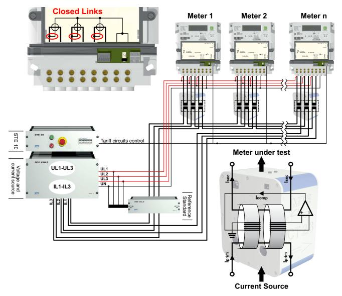
In meter testing stations, dangerous voltages above 50V AC might be available. The user must be protected from them. Following measures secure and enable a voltage separation:
