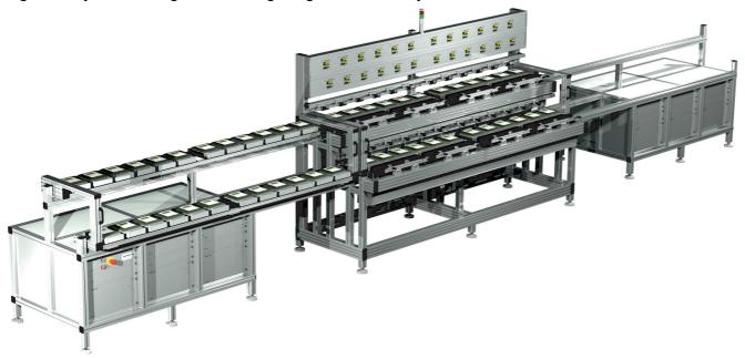
Gantry systems on trolleys are used, if many special or different single- and three-phase meter types require a quick and flexible adaptation in the test procedures. Whilst the test is running other trolleys can be used in parallel to perform the assembly, preheating and if required meter isolation test. That guarantees the user an ongoing throughput.
