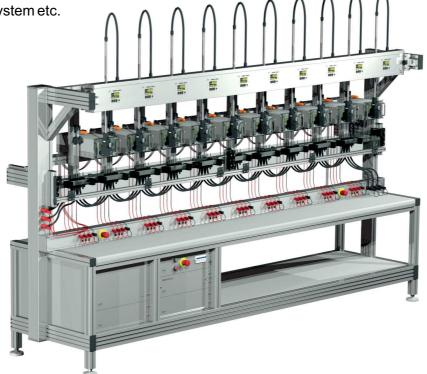
This picture shows a meter test rack with total 10 measurement positions for 10 bottom connected DIN meters or 10 chassis meters.
